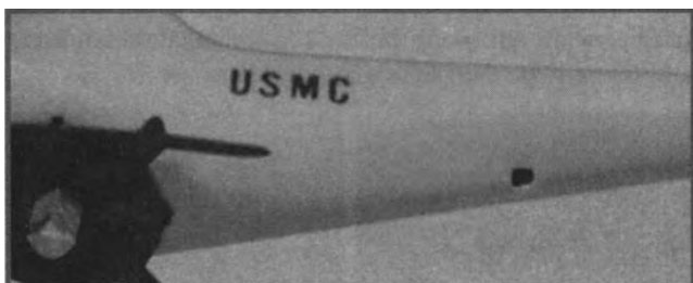
(Above): All original USMC helicopters have a tapered hole.
