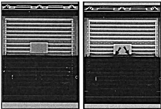
(Left): On an original, the masked line is almost straight across the top, and small amounts of leakage or bleeding can be seen. (Right): The masking on a fake is a dead giveaway.
