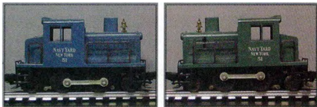
Fig. 36 (Left): This side of an original 51 Navy switcher spent the summer in a child's sandbox. (Right): This side faced the sun.
