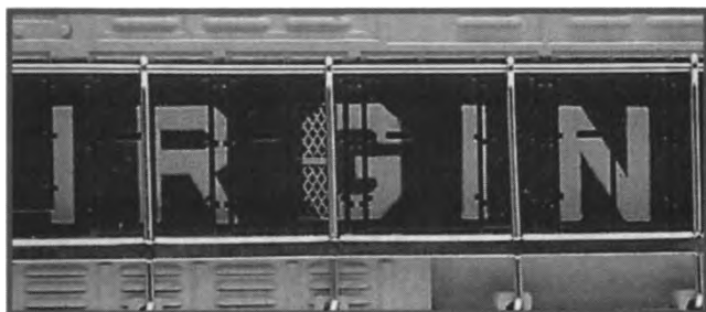
The left side of an original letter "G" rests on top of the vent, showing some space in between. The "G" is also interrupted by the door panel lines. The repainted "G" covers the vents and door panel lines.
